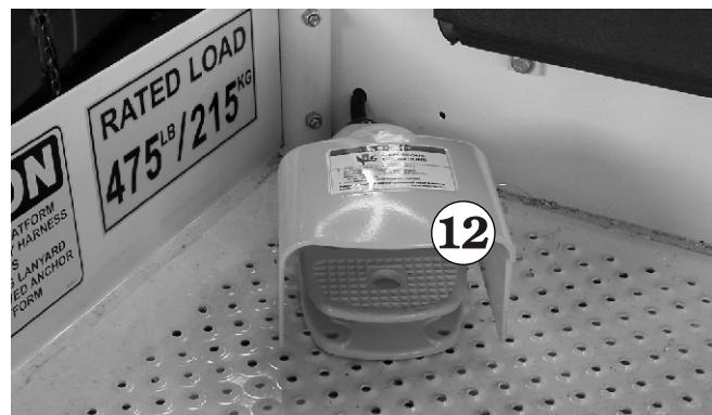
Figure 6.6 - Upper Controls - Foot Switch
