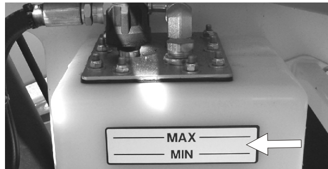
Figure 7.8 - Hydraulic Oil Level
