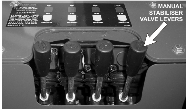
Figure 6.7 - Stabiliser Controls (Manual)
