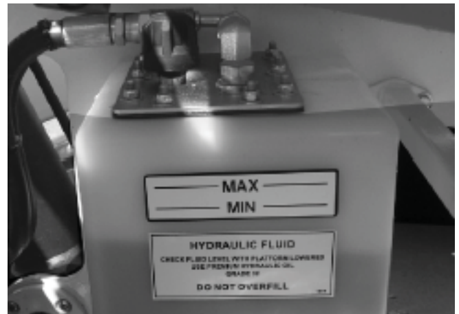
Figure 4.3 - Hydraulic Oil Level
