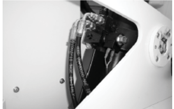
Figure 9.6.1 - Manual Lower Valve, Lower Boom
