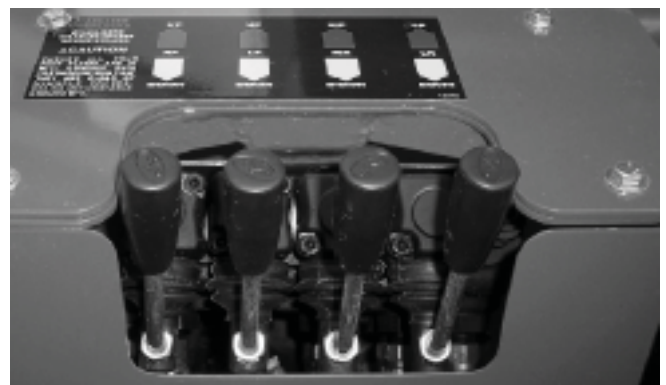
Figure 6.7 - Stabiliser Controls (Manual)
