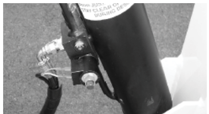
Figure 9.6.2 - Manual Lower Valve, Upper Boom
