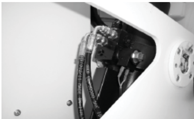
Figure 6.3 - Ground Controls, Emergency Bleed Down Control Valve, Lower Boom
