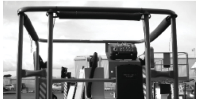
Figure 7.17 - Platform Gravity Gates
