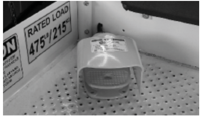
Figure 6.6 - Upper Controls - Foot Switch
