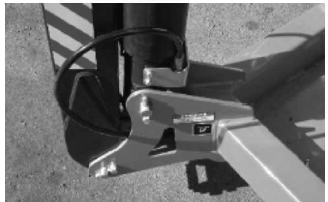
Figure 10.4 - Tie Down Lugs
