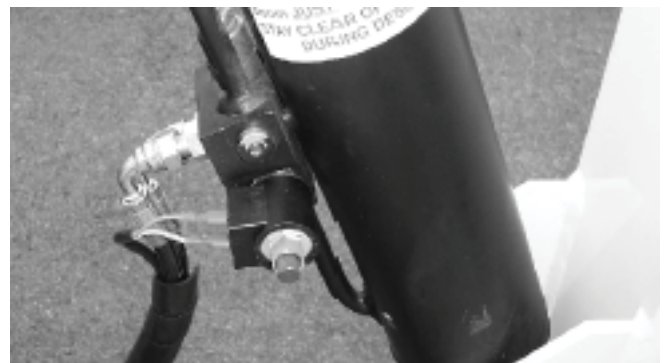
Figure 7.21.2 - Emergency Lower Valve, Controlling Upper Boom
