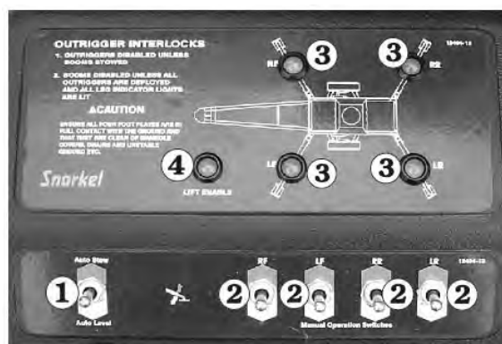
Figure 6.11 - Self Leveling Stabiliser Controls
